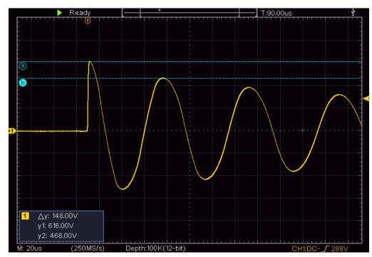
The following oscillograms show the damping factor verification for a 600 V transient.
