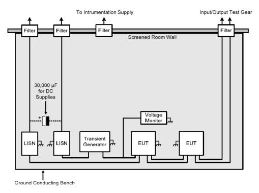
[1] The indicated voltage will determine which pulse output to connect the EUT to. This will be either 600 V, 750 V or 2500V.
